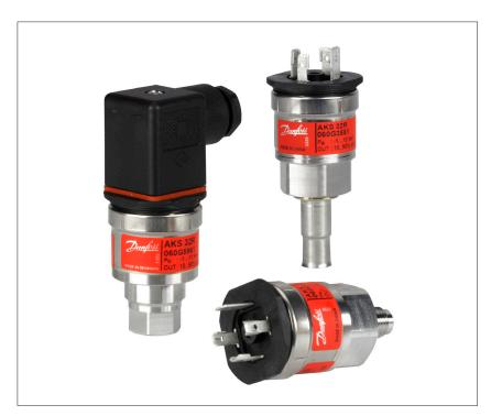
AKS 32R is a ratiometric pressure transmitter that converts the measured pressure to a linear output signal. The min. value of the output signal is less than 10% of the actual supply voltage. The max. value is more than 90% of the actual supply voltage.
